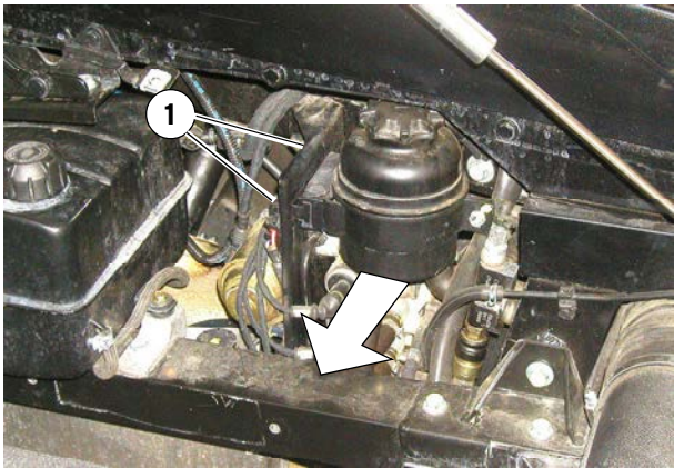
Fig. 1 Screws of the e-gear hydraulic tank slide
